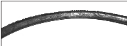
Shining surface due to high slippage
